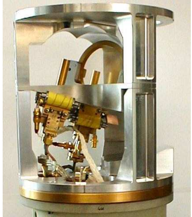
Figure 1: A view of the upper part of the prototype cartridge, comprising the cold optics and two 2SB assemblies. The two horns are staring into two elliptical mirrors machined into the roof of the assembly, while a third mirror, partly hidden at the right, couples the cartridge to the telescope optics. The polarization diplexing grid (round frame) can also be seen.
