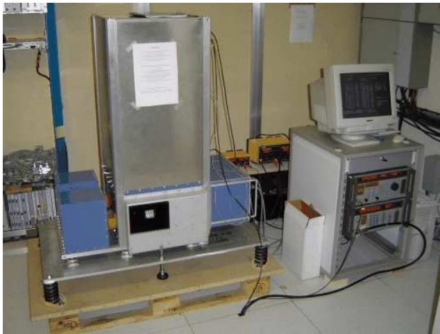
Figure 3: The EFOS-1 maser in the PdBI correlator room. The maser itself is mounted on two stages of shock absorbers, which protect the frequency standard during its transport by road and helicopter. Its power supply can be seen in the background. To the right, the rack with the frequency synthesizers is installed, together with the computer which monitors the operating parameters of the maser.
