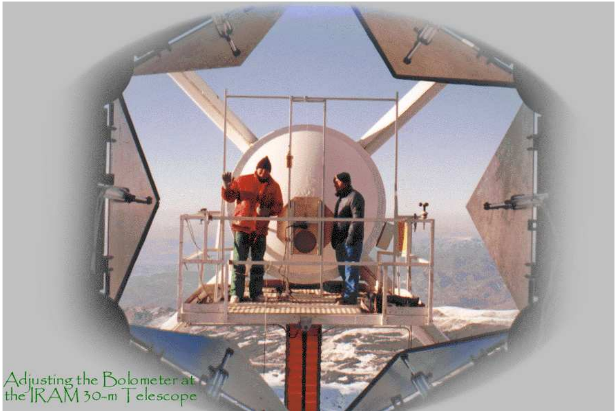
Aligning the bolometer at the IRAM 30-m Telescope: A view from the receiver cabin through the vertex windows shows two engineers adjusting the beam of the MPI bolometer for the winter 1999/2000 campaign. The mechanism on the platform allows to move a chopper wheel (pointing at an ambient load and the sky) in horizontal and vertical direction. The optimum alignment is achieved when the bolometer looks toward the center of the subreflector. With this picture the IRAM staff send their Christmas greetings and best wishes for the year 2001.
